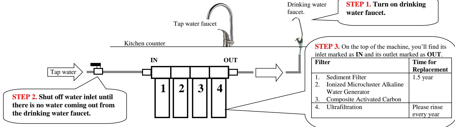
**STEP 4.** Each stainless steel cylinder is full of water. Disconnect the system and put it inside a sink, or place a bucket and a towel under the stainless steel cylinder to prevent water from spilling.
