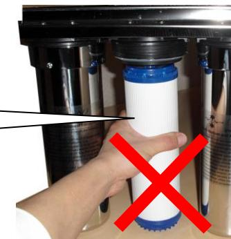
**Grab the top of the filter cartridge and pull it off. Then replace it with the new filter cartridge.**
